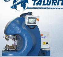
Arm (option) for T-PANEL (option) mounted on a one pillar P 0600T 1S.
